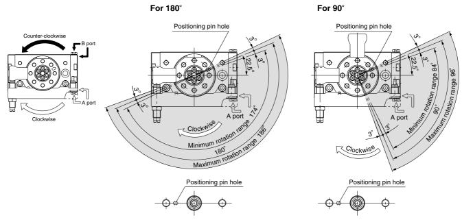
Position of bottom positioning pin hole
