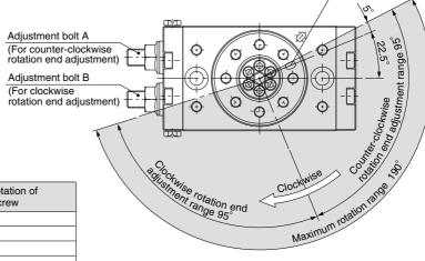
With adjust bolt, internal shock absorber
