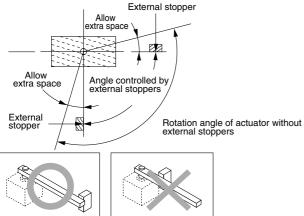
External stopper becomes a fulcrum, and load's inertial force is applied to shaft as bending moment.
